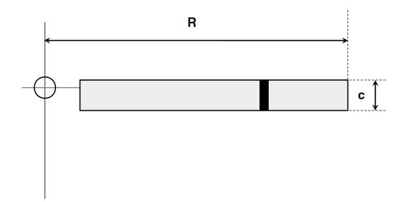
*R*: propeller radius *c*: propeller chord
