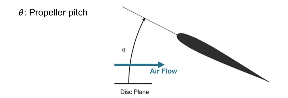
What direction is the force if the leading edge is LOWER than the trailing edge?
