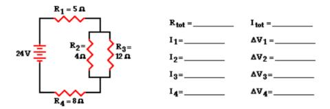
(b) Given the following circuit diagram use the concept of equivalent resistance to determine the resistances marked unknown. <u>Show your calculations.</u>
