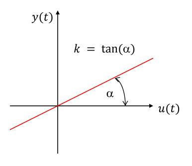
Static characteristic (for static linear systems it is a straight line).
