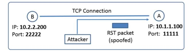
**Goal:** To break up a TCP connection between A and B. **Spoofed RST Packet:** The following fields need to be set correctly:
