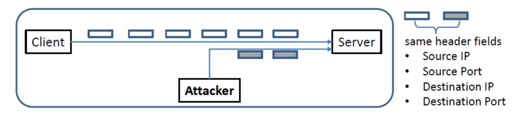
**Goal:** To inject data in an established connection. **Spoofed TCP Packet:** The following fields need to be set correctly:
