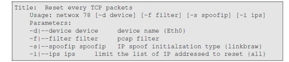
Using netwox tool 78, we can generate a spoofed RST packet to the client or server. If the attack is successful, the other end will see a message "Connection closed by foreign host" indicating that the connection is broken.
