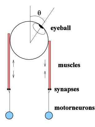
$J\ddot{\theta}(t) + B\dot{\theta}(t) + K\underbrace{\theta(t)}_{\text{output input}} = \underbrace{\tau(t)}_{\text{input}}$ J, B, K – parameters
