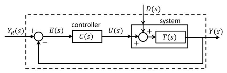
Let us calculate the transfer function. Keep in mind that this is a MIMO system, as there are two inputs ( $Y_R$  and D) and one output (Y).
